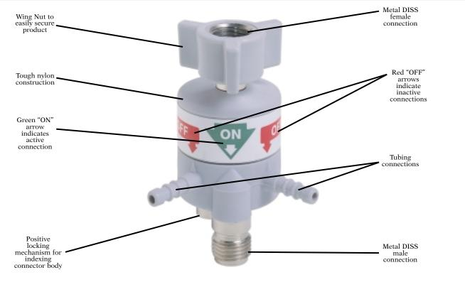
NOTE: The Flow Selector is a selectable single flow device. Flow is only delivered to the selected connection indicated by the 💜 arrow. No flow is delivered to the connection indicated by the 🕶 arrows.
