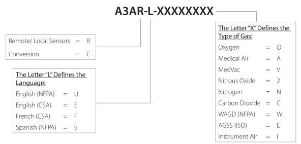
**Example:** 3 Gas LCD Alarm Consisting of Oxygen, Medical Air & Vacuum = **A3AR-U-OAV**
