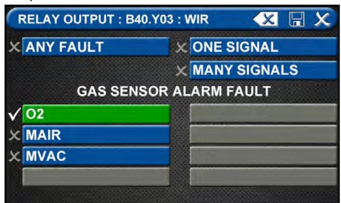
Figure 117: Gas Sensor Alarm Fault
