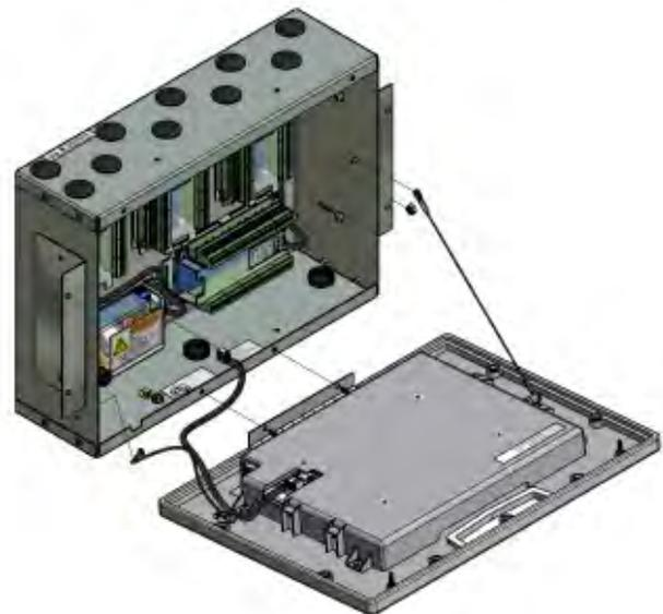
Figure 29: Attach Front Panel and Lanyard
