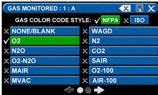
Figure 80: Gas Monitored Tab
