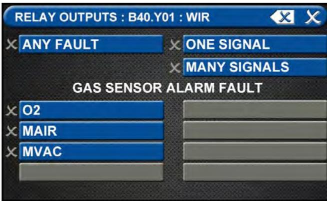
Figure 114: Relay Output Signals Screen
