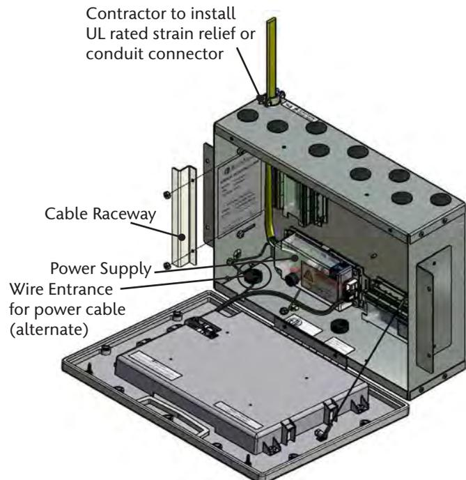
Figure 20: Wire Routing
