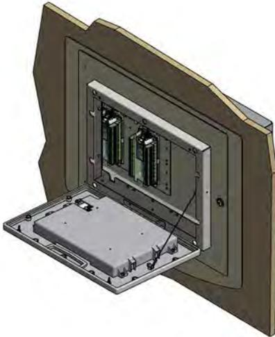
Figure 133: MEGA3™ Double Mount Front Panel Assembly
