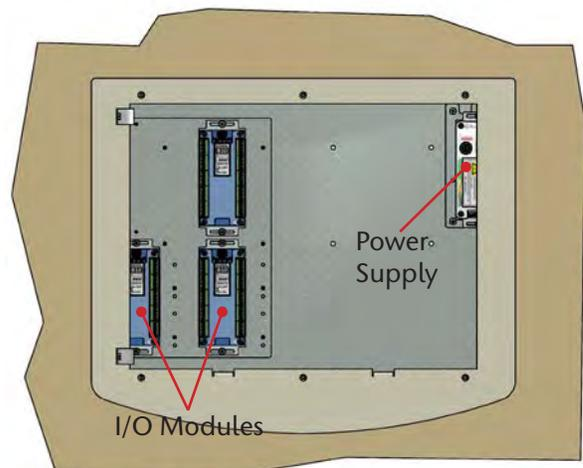
Figure 129: Double Module Positions
