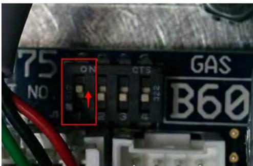
Figure 123: DIP Switch Setting
