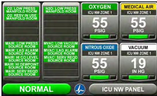
Figure 38: Combination Alarm Main Screen
