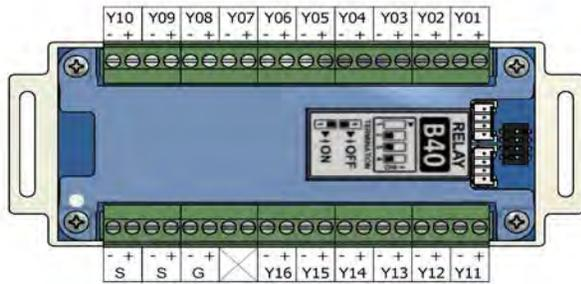
Figure 6: B40, B41, B42, B43 Relay Output Board
