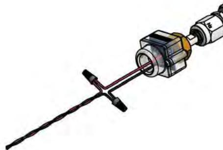
Figure 31: Remote Sensor Module Connection
