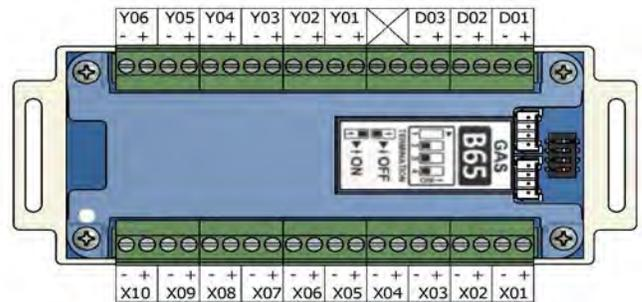
Figure 9: B65 Gas Combination 3D, 10X, 6Y Board
