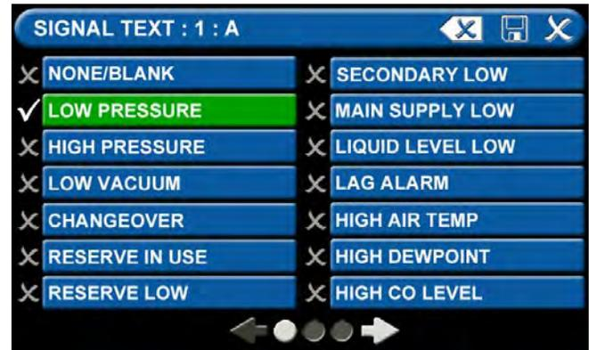
Figure 81: Signal Settings Tab
