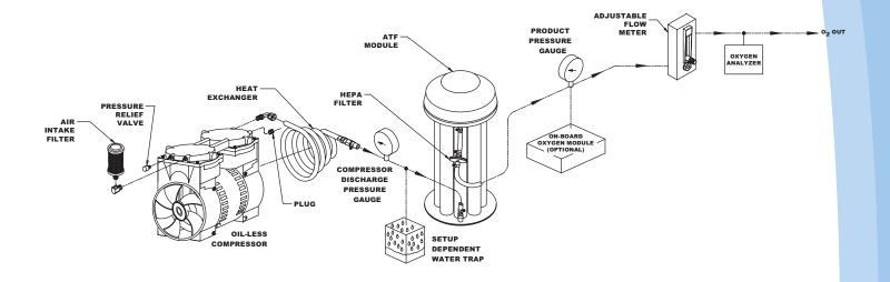
AirSep excels as the leading supplier of PSA oxygen systems — worldwide — offering the most cost-effective, most efficient, and safest oxygen sources for today's diverse oxygen applications. The ATF module is the main component of a PSA system. When matched with the proper equipment, the ATF can deliver a reliable flow of oxygen to any application.
