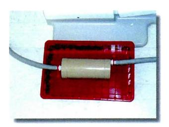
The chair side filter/amalgam separator will need to be changed when vacuum levels fall below recommend values (see the manual for additional details). The used filter (still connected to vacuum lines) should be placed in a tray that will collect any spilled wastewater, preventing it from contacting the operatory floor.
