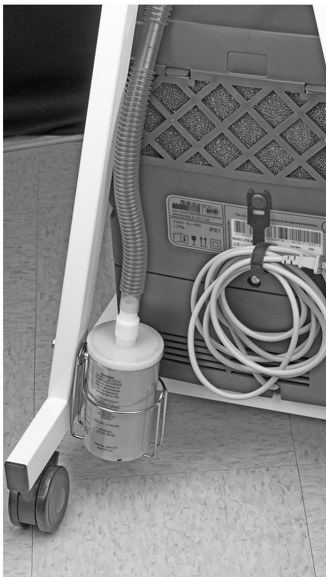
Optional F-Air evacuation kit P/N EVC555 (Shown on M6000)
