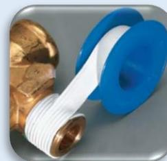
We offer our **MercO M45 Threadmaster® Perseus™ High Density Threadseal Tape** in industry standard ½ inch, ¾ inch, 1-inch widths and 520 inch and 1296-inch lengths. Unlike the new, gimmicky kid on the block ours has no coloring added to degrade purity. 100% *pure* virgin PTFE. Higher density at .80 g/cm<sup>3</sup>. Made in ISO 9002 certified facilities to meet UL, ULc requirements and Mil Spec T-27730A. Labeled on both sides with branding, UPC and instructions for use.
